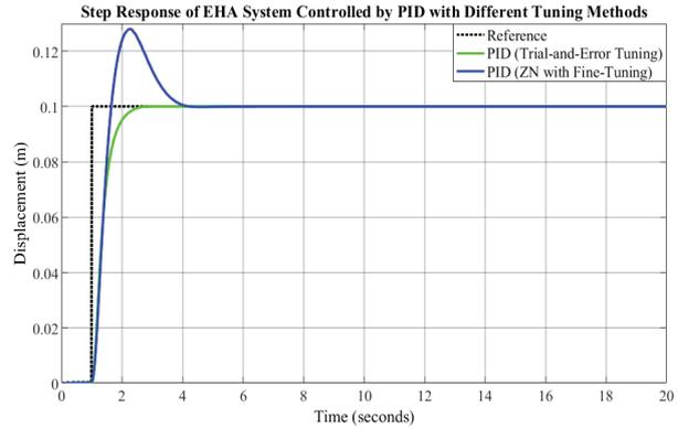
Figure 3 Step response of designed PID control systems
