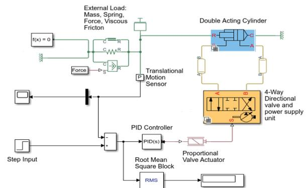
Figure 1 EHA model in MATLAB Simulink
