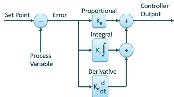
Figure 2 PID controller in parallel algorithm
