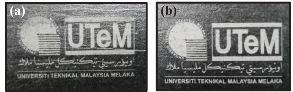
Figure 4 (a) Marked surface at 4 W and 2000 mm/s (surface roughness 3.9 \mu\text{m} ) (b) Marked surface at 12 W and 500 mm/s (surface roughness 10.2 \mu\text{m} )
