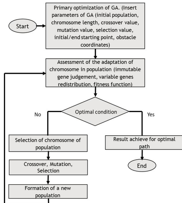
Figure 1 Flow chart of GA for mobile robot planning task
