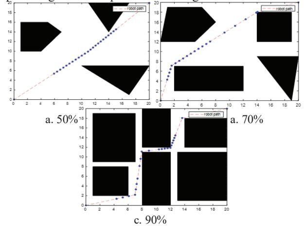
Figure 3 Mobile robot path with various percentages of obstacle
