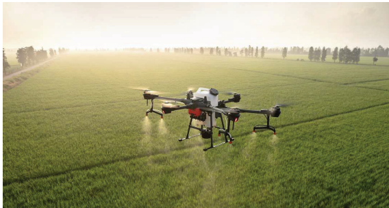
Fig 3: Crop spraying heavy lift multirotor drone
