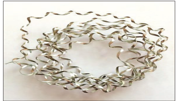
Figure 3 Continuous chip formation
