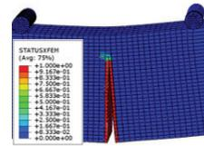
Figure 2: Crack growth tracked from XFEM model
