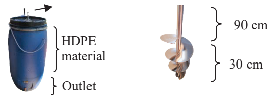
Figure 1: a) Compost bin from HDPE materials, b) Stainless steel shift blade
