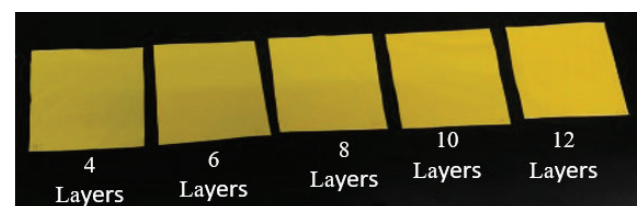
Figure 1: Geotextile sample with different layers of LDPE plastic; (a) 4 Layers, (b) 6 Layers, (c) 8 Layers, (d) 10 Layers and (e) 12 Layers
