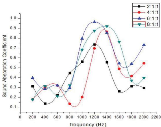
Figure 3.1: Result of Sound Absorption test of difference ratio of HDPE plastic waste with polyurethane foam
