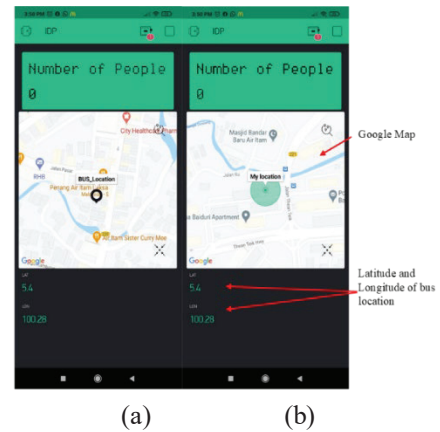
Figure 4 Mobile phone application: (a) Location of the bus, (b) Location of the user
