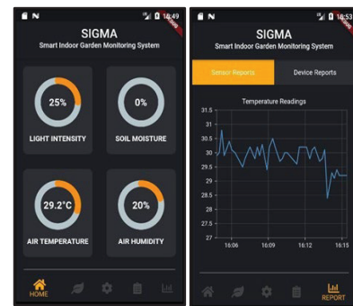
Figure 2 (a) Sensor's data visualisation (b) Time-series report of sensors value
